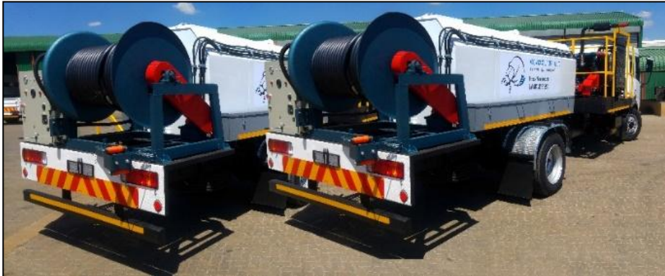
Large sewer jet machine working
