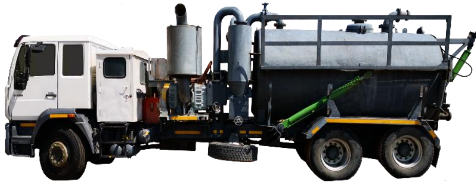
Silt and sludge being removed from sewer pump stations and large septic tanks.
